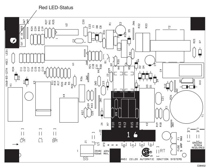
Fig. 38 - Integrated Gas Control (IGC) Board
